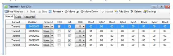
By selecting the Transmit button, the corresponding message is sent to the keyboard. The button then changes the color.
