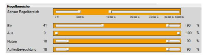
E.g. A Sensor Range of 5000lx - 10000lx is set. That means: 5000lx corresponds to a value of 0d and 10000lx of 255d on the CAN bus.
