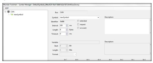
Bus: Indicates on which CAN-Bus the settings are made.
