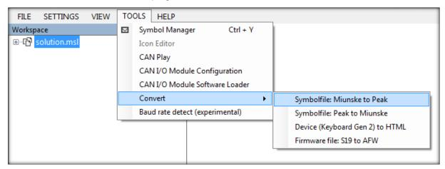
Symbol Manager Window to configure CAN-messages. More Informations in section Symbol Manager Icon Editor Tool to create new icons Tool to create artificial CAN-Bus traffic **CAN Play** CAN I/O Module for the I/O Module exist two programmer adapter. You need this if you have Configuration a blue box. CAN I/O Module for the I/O Module exist two programmer adapter. You need this if you have Software Loader a blue box. Convert Here you can find various programms to convert between fileformats
