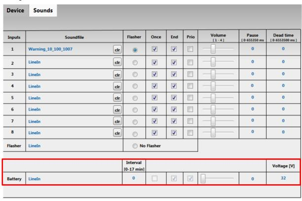
In the row "BATTERY" a sound file and then the voltage limit is selected at which this sound should be played back.
