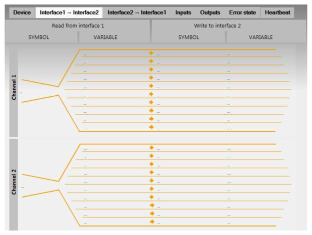
Clicking on a variable ("...") in the left part of the table ("Read from interface 1") opens the Symbol Manager. Then a variable for the previously selected CAN-Bus has to be defined in the Symbol Manager.
