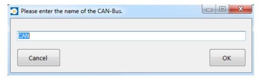
If the name of the CAN-Bus is given, it has to be confirmed by clicking the "OK" button. After confirming, a new input field for the description appears.
